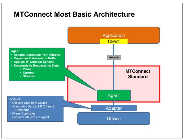
Figure 1 – MTConnect Basic Architecture
